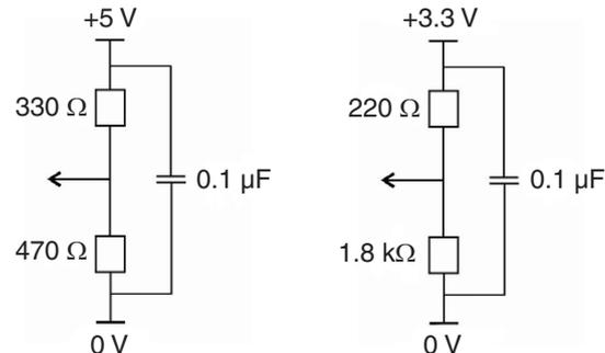
**Figure 5 – Examples of passive bus terminations**
