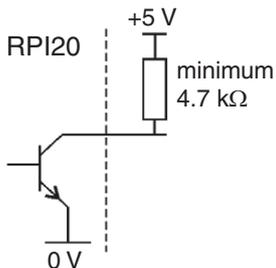
**Figure 7 – Open collector error output wiring**
