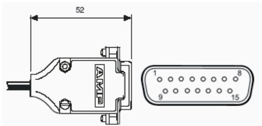
**Figure 4 – Analogue quadrature input mating connector (15 way D-type male connector)**
