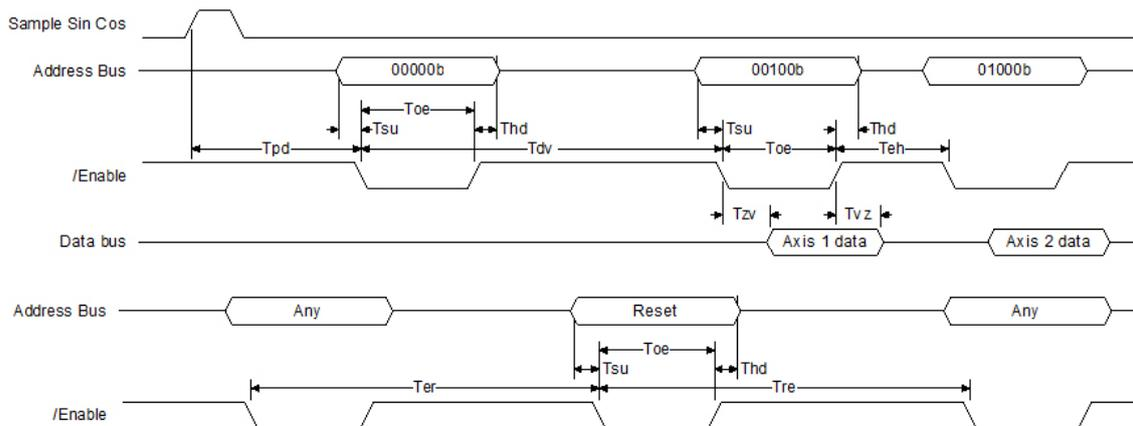
Figure 8 – RPI20 parallel bus timing diagram
