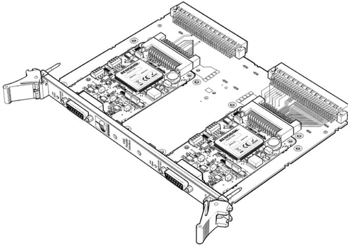
**Figure 3 – Two RPI20s in a VME host PCB**
