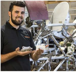
Renishaw produced the metal brackets from aluminium powder in four separate builds using one of its AM250 additive manufacturing machines.
