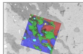
Figure 3e. A Raman image overlaid upon the SEM-BSE image of the same geological sample
