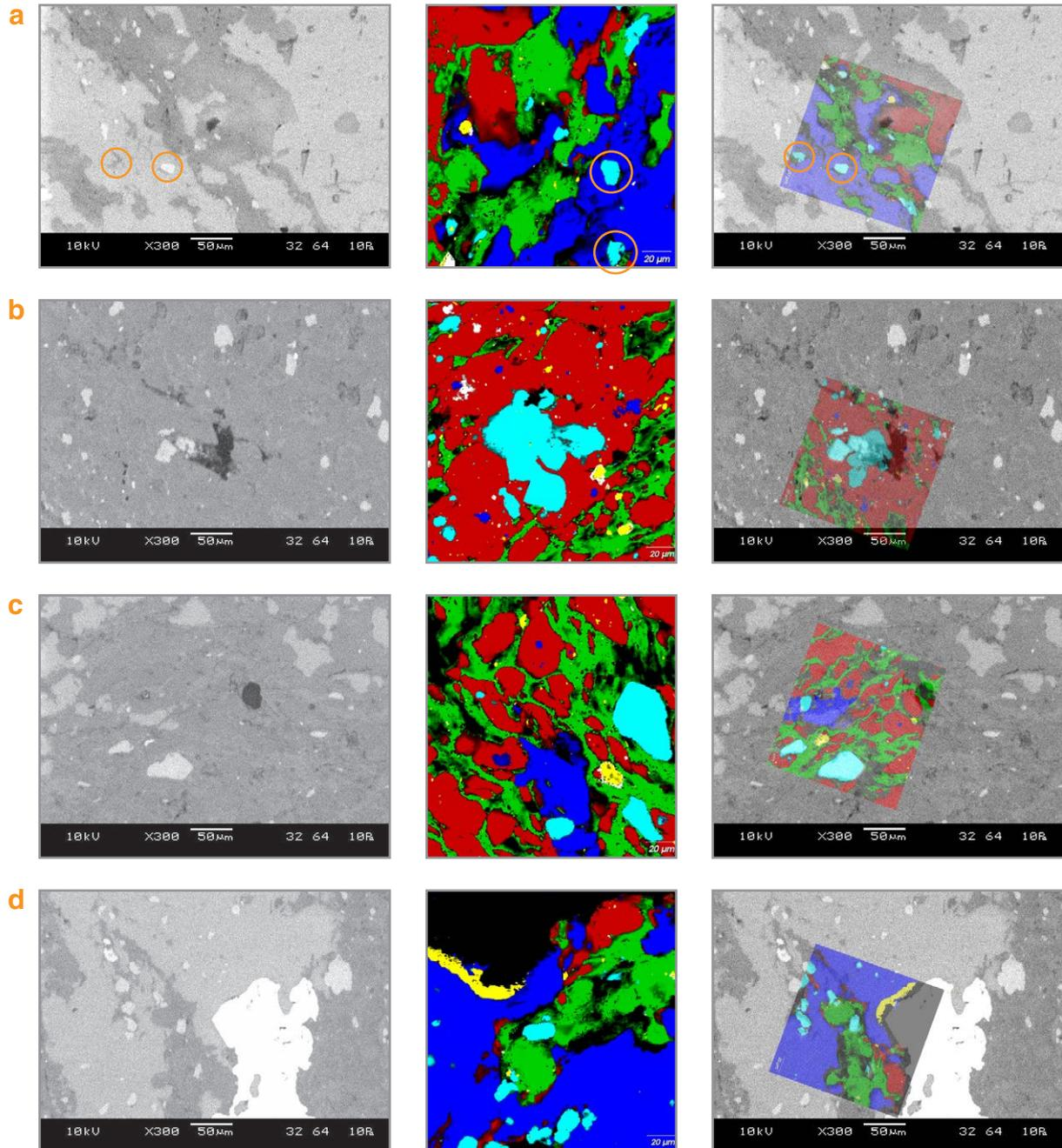
Figure 4. (L to R) SEM-BSE, Raman, and overlaid SEM and Raman images acquired at four positions (a to d) on the geological sample. The colours in the Raman images correspond to the identified components: rutile (yellow), anatase (white), apatite (light blue), carbon (green), quartz (red) and calcite (dark blue)
