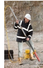
Compact laser scanner maps underground voids
