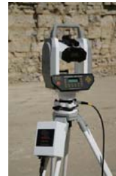
Laser scanner maps a quarry face
