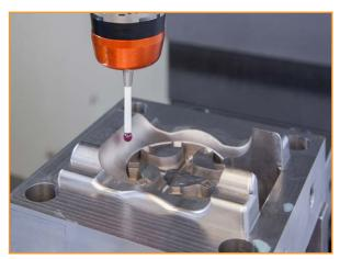
In-cycle probing with a Renishaw Primo Radio Part Setter on an XYZ high-speed vertical machining centre.
