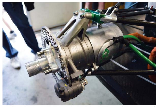
Optimised wheel carriers in a titanium alloy made via Renishaw's additive manufacturing process saved a total of 1.5 kg in vehicle weight.
